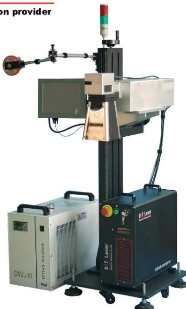
Datang UV laser marker is specially used for marking of pipelines.
