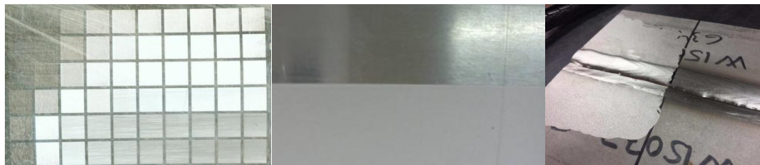
a 铝合金焊前焊后激光清洗
