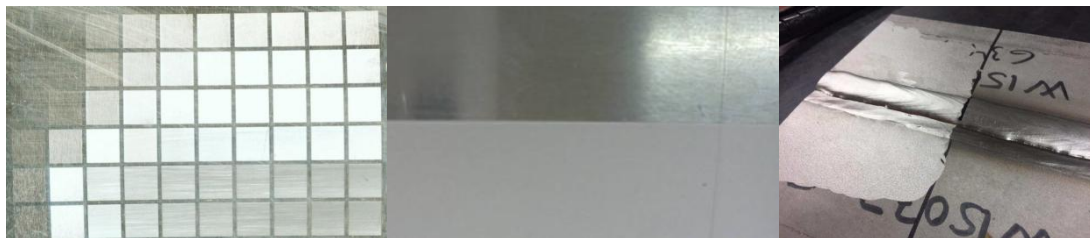
a 铝合金焊前焊后激光清洗
