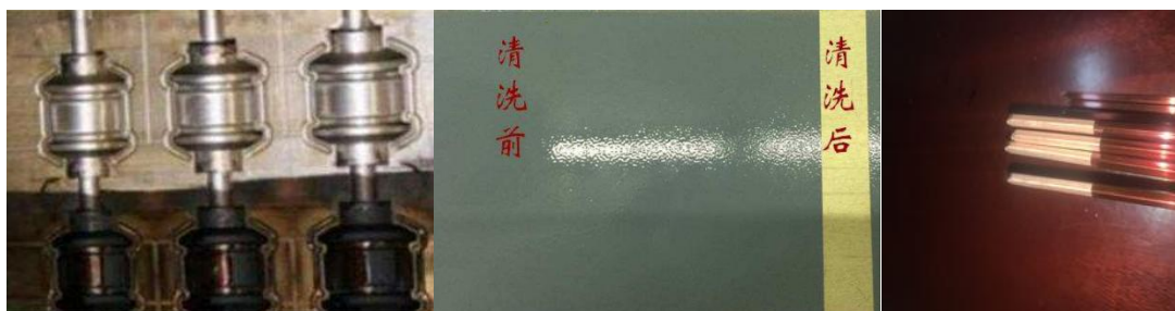
c 激光清洗油污、油漆
