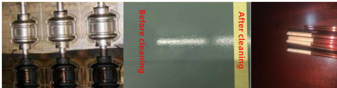
c Laser cleaning of oil and paint
