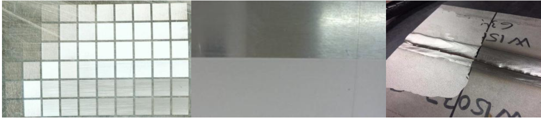
a Laser cleaning of aluminum alloys before and after welding
